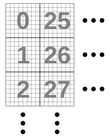
By lining the characters into vertical columns like this, advancing vertically by one pixel adds a constant 8 bytes each time, as shown below:
