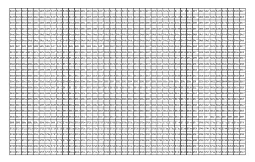
That is, each character cell uses one byte of screen RAM, and the addresses increase smoothly, both within lines, and between lines. Super-Extended Attribute Mode requires two bytes per character cell. So if you set \$D054 to \$05, for example, you will get screen addresses like this:
