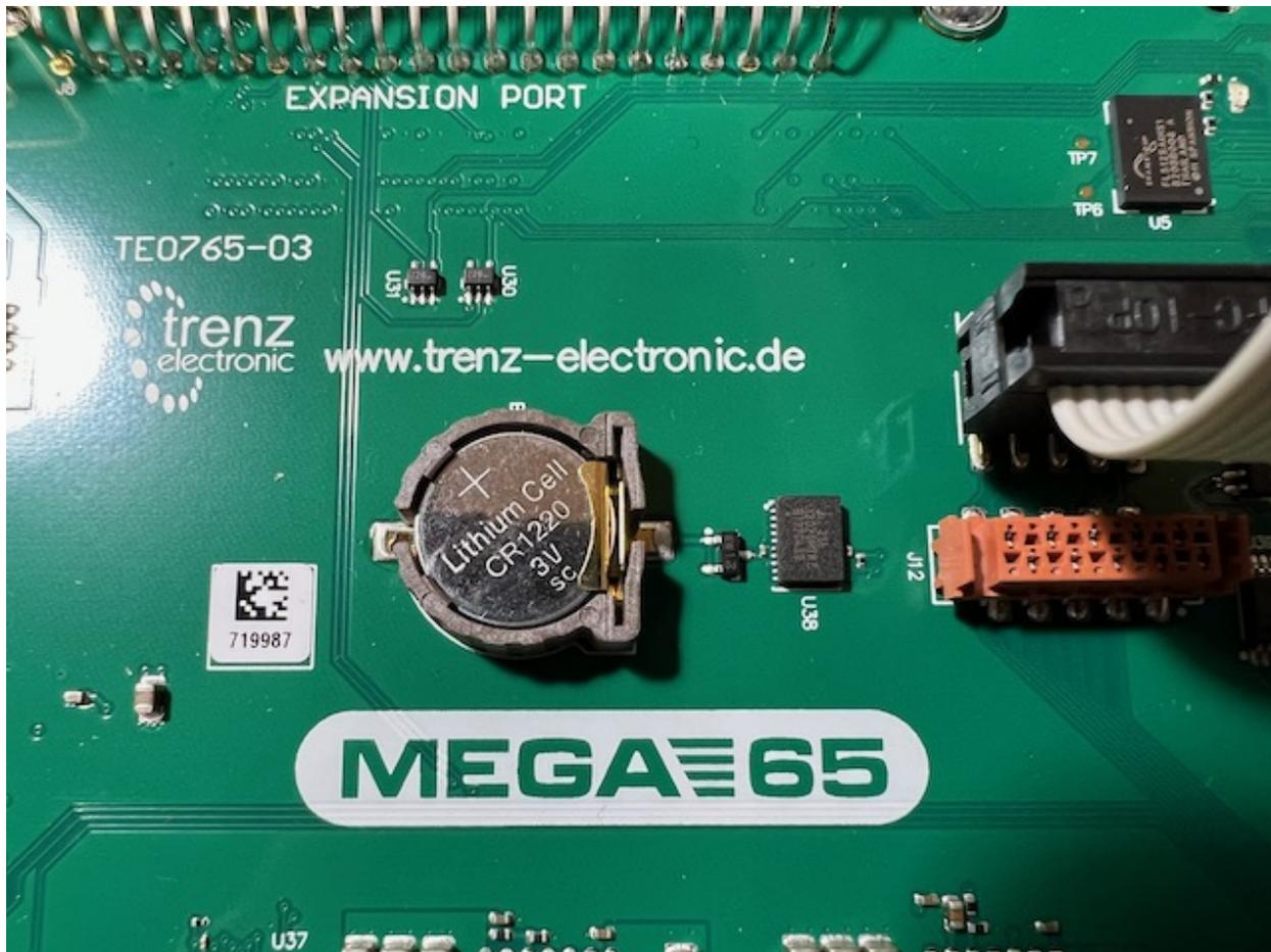
Install the CR1220 battery. Locate the battery holder on the main board. Insert the battery under the tab, with the positive (+) side facing upward. Push down to secure it.
