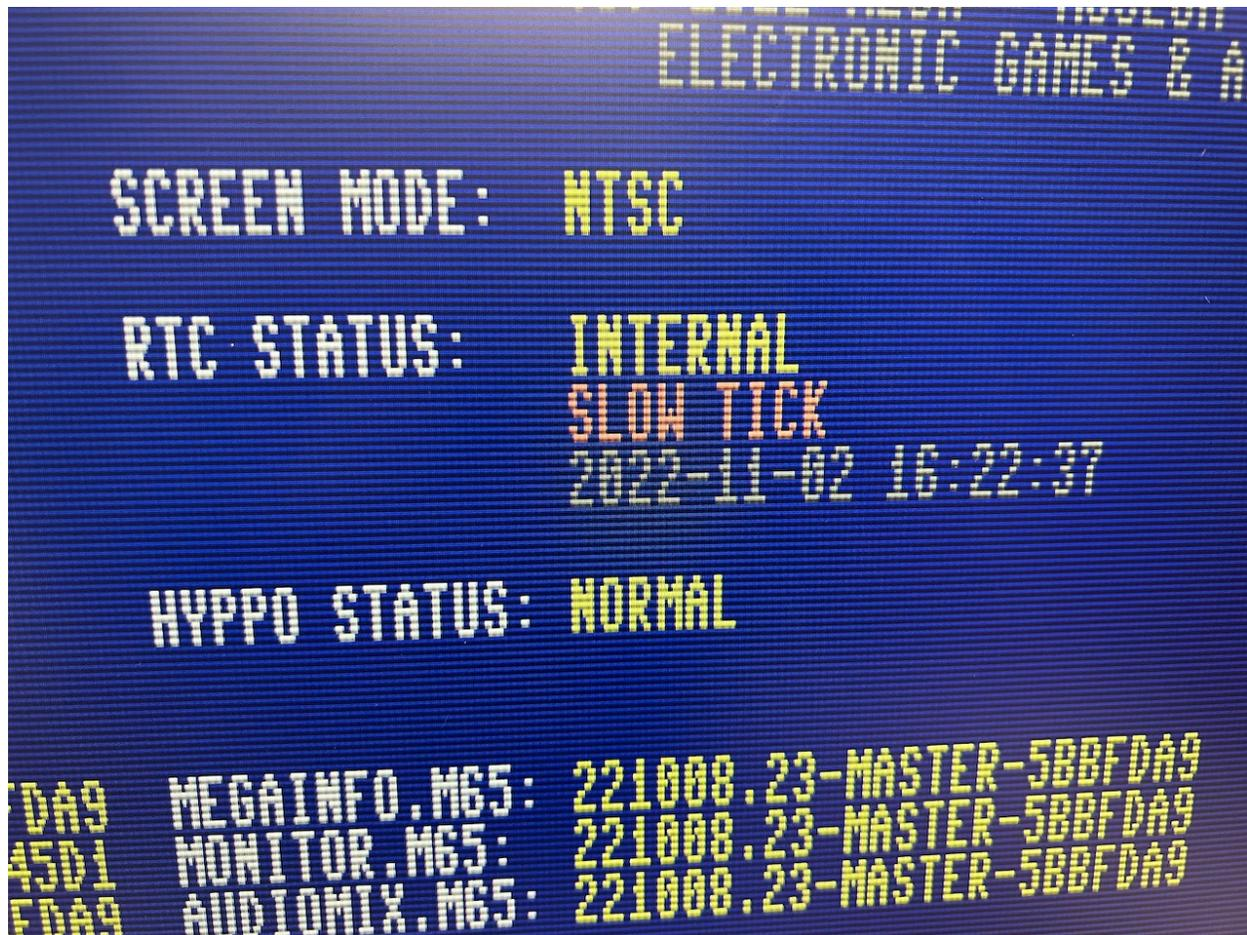
After installing the Grove (“external”) RTC, MegaInfo reported a working clock:
