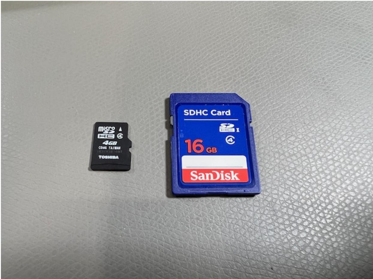
MEGA65 only uses one SD memory card at a time. If there is a microSD card in the external slot, it ignores the full-size SD card in the internal slot. The SD card contains the operating system software (“ROM”), firmware (“core”), the system utilities (such as the Freeze menu), and D81 disk images.
