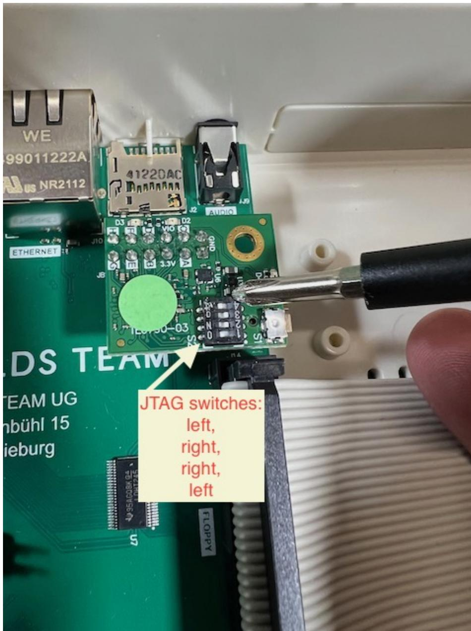
Connect a mini-USB cable to the JTAG connector, and run the cable out the back of the MEGA65 case. You can feed it out the cartridge port (potentially blocking access to the port), or punch out one of the unused port covers in the back case. Connect the other end to your PC.
