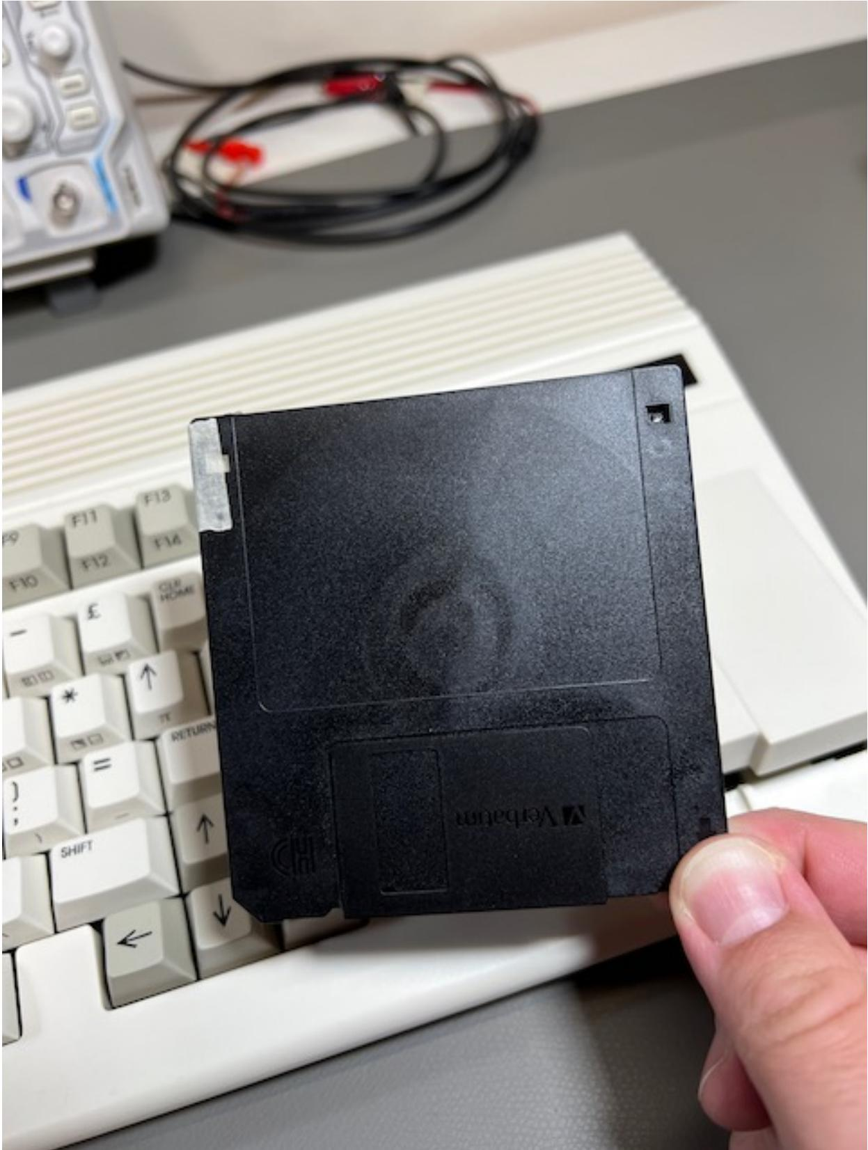
**Tip:** Until this is fixed in a future software update, an HD disk with the hole exposed will not work with the MEGA65. If your disk isn't working, double-check that the hole is covered.
