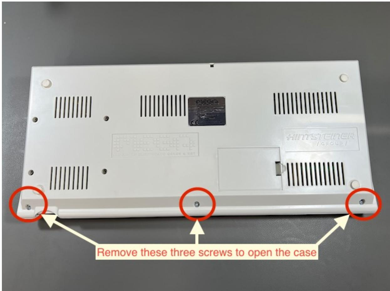
The case separates into a top piece and a bottom piece. The keyboard is attached to the top, while the disk drive, ports, and main board are attached to the bottom. The keyboard is connected to the main board with a ribbon cable.
