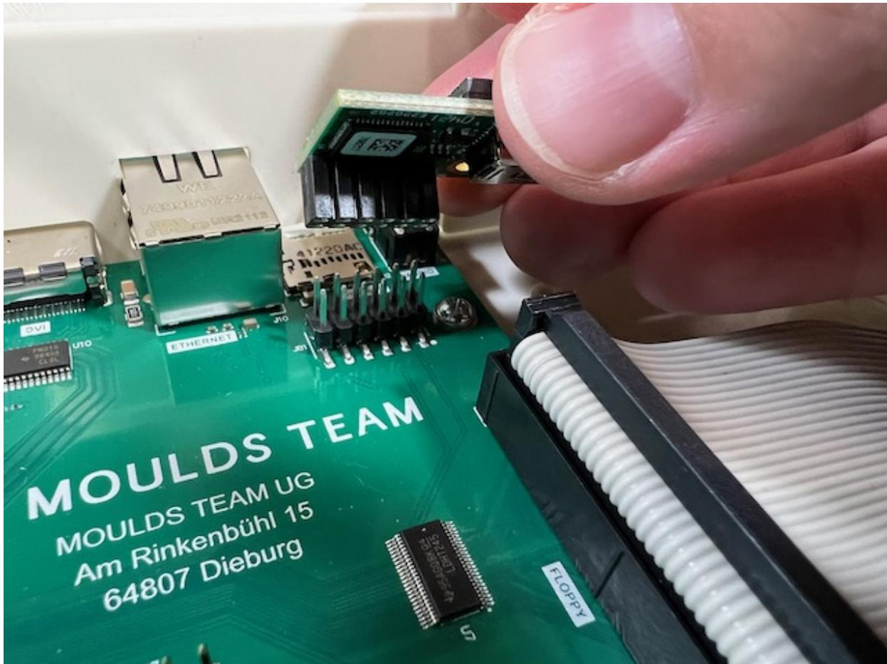
Use a pin or a small screwdriver to set the DIP switches on the connector to left, right, right, left, as shown. This configures the adapter to draw power from the USB connection. (Other documentation suggests left, right, left, right, which draws power from the MEGA65. The USB setting worked fine for me.)
